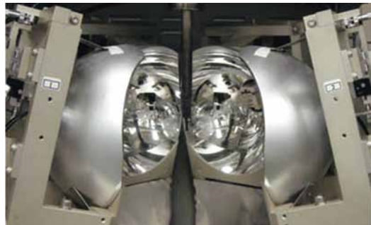
傾斜鏡型赤外線集中加熱炉 Tilting Mirror Type Infrared Convergent Image Furnace
